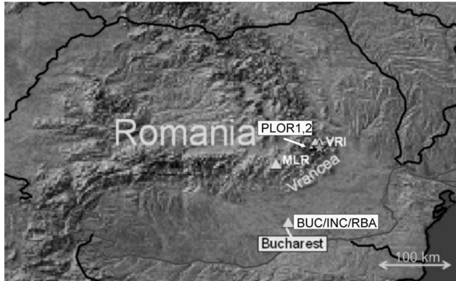
Figure 1. Distributions of strong motion sensors in the Romanian EEW system and additional stations used for the definition of scaling relations. The star indicates the location of the October 27, 2004 Vrancea earthquake ( M_w = 6.0 ).
