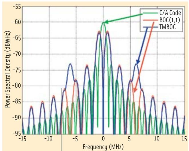
**FIGURE 3** Unit Power PSD of L1C Pilots using BOC(1,1) and TMBOC Spreading Modulations, Compared to C/A Code PSD, Showing the Increases in Beneficial High Frequency Power
