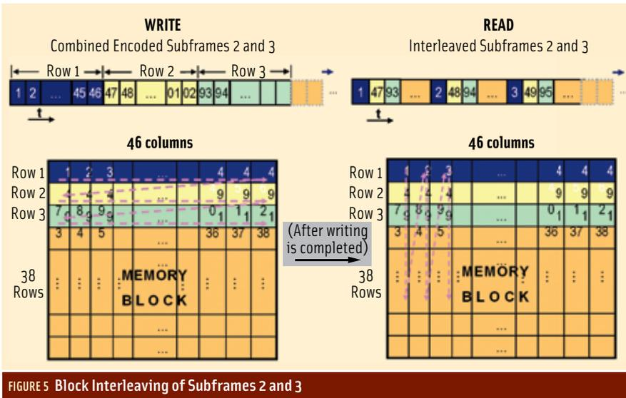
FIGURE 5 Block Interleaving of Subframes 2 and 3
