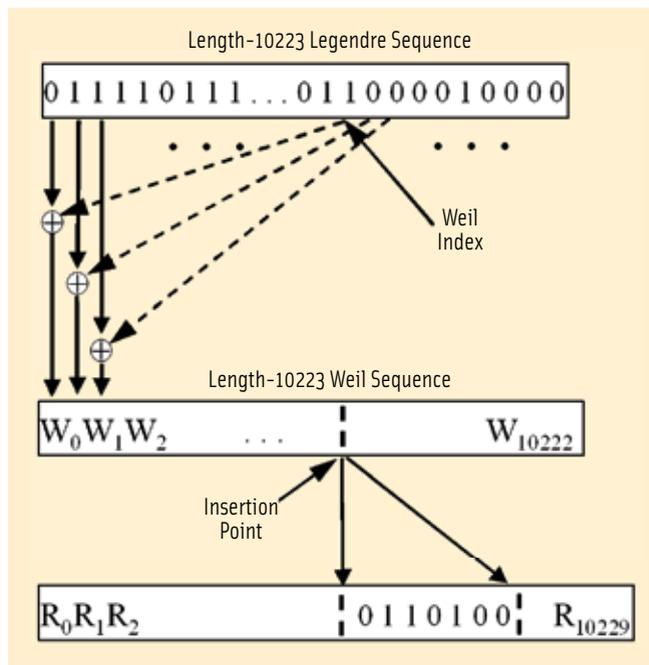
**FIGURE 2 Construction of Length-10230 Weil-Based Spreading Codes.** The figure shows construction of Weil Sequences from a single Legendre sequence, then extension to 10,230 bits by inserting seven additional bits, all using simple logical operations.
