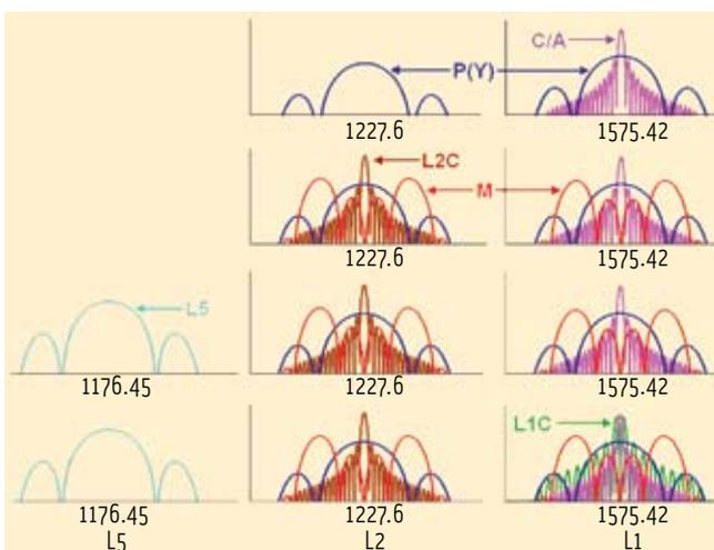
FIGURE 1 Evolution of GPS Signal Spectra (from top): Original, Block IIR-M, Block IIF, Block III
