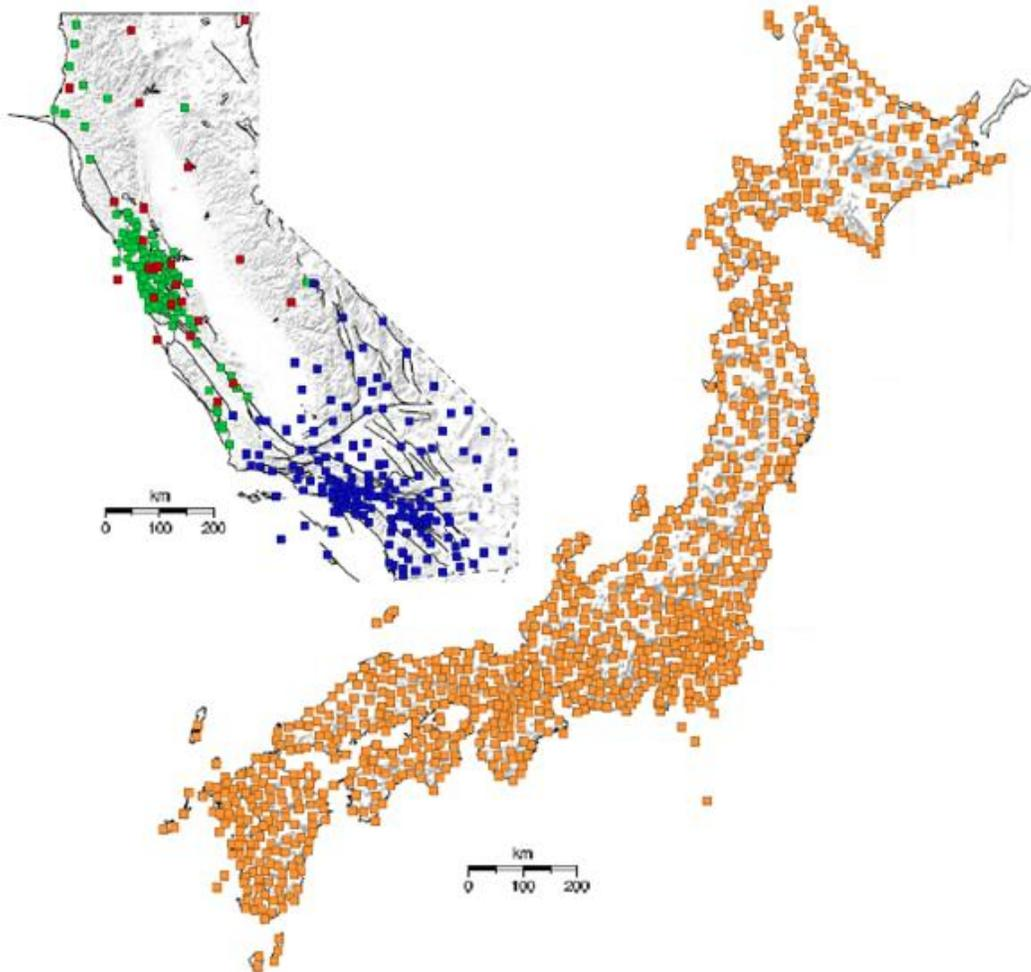
*Figure 2: Earthquake sensor density: California versus Japan. New sensors need to be added in California to shorten the CISN sensors spacing to approximately 12 miles to facilitate timely EEW. The shorter the station spacing, the smaller the blind zone will be because warnings can be issued faster.*
