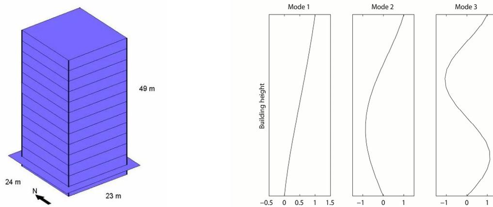
Figure 1. (Left) *SketchUp* visualization model of 12-story concrete building used in analysis. (Right) First three NS translational mode shapes resulting from the Timoshenko beam calculation for the 12-story concrete building.
